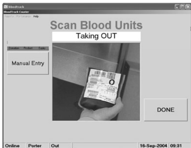
Fig. 1. Blood collection with BloodTrack Courier. The bar code of the unit is scanned, bringing up the patient details on the screen. A verbal prompt asks the member of staff to ensure that the blood was for the correct patient by checking the patient identification details on the blood collection slip match those on the screen.
